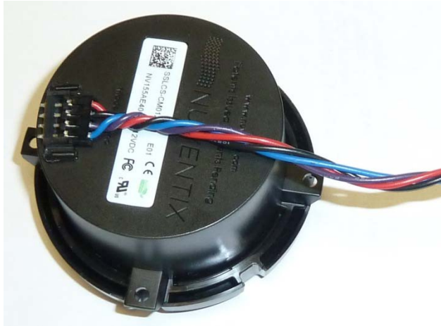
Figure 6 - SynJet Cooler with WALS Cable Attached
