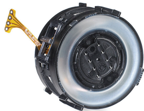
FIG. 3. Synthetic jet engine with oscillating diaphragm.
