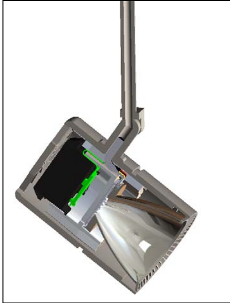
Figure 9: Attachment to the Center Perimeter Heat Sink Hole
