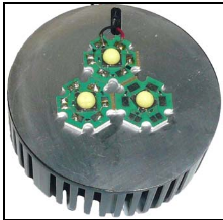
Figure 8: Heat Sink Face with LEDs Attached
