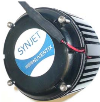
Figure 5: Running SynJet PAR20 LED Cooler Power and Control Wires
