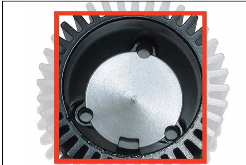
Figure 4: Partially Blocked Heat Sink Channels
