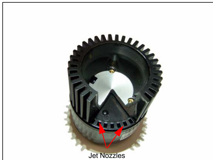
Figure 2: SynJet MR16 Nozzles
