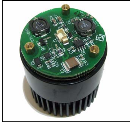
Figure 12: PCBA Mounting Features
