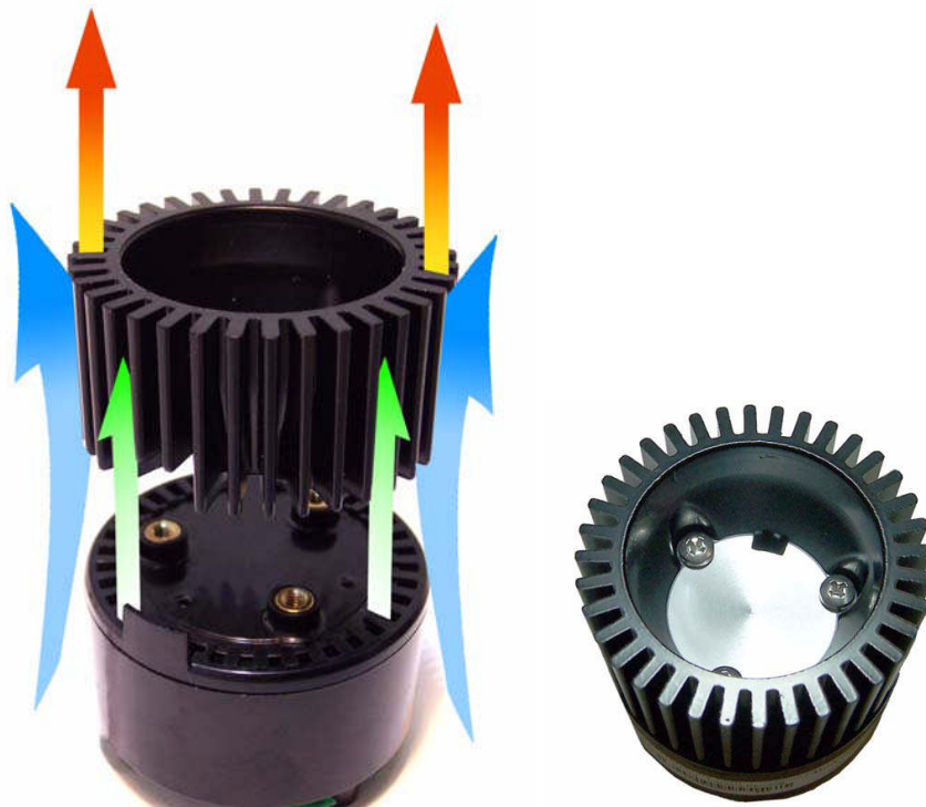
Figure 2: MR16 SynJet® cooling module with heat sink (left). This model is designed for up to 20 W applications. Arrows indicate air flow. Green for pulsating SynJet flow, blue for entrained ambient air, orange/red for rejected heated air from heat sink. Right: LEDs are installed on inside heat sink surface.
