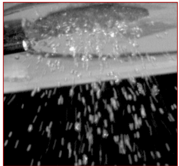
Figure 10b. Ejected secondary droplets with the atomizer in a downward-facing horizontal orientation. The supply tube is tangential to the atomizer.
