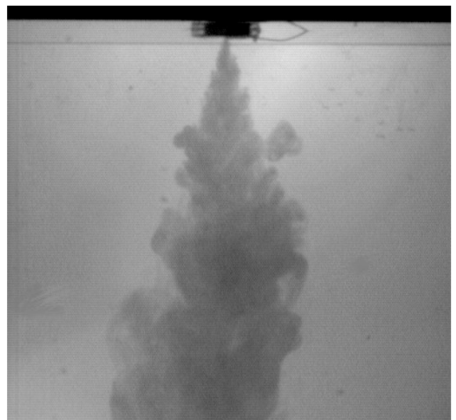
Figure 3. Dye visualization photograph of the VIBE turbulent jet. The dye is entrained radially from an injection port near the edge of the diaphragm.
